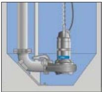
The TOPS sump design creates turbulence that re-suspends solids, dramatically improving solids transport.
