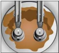
Sludge and solids in the conventional sump have been deposited across the entire sump floor.
